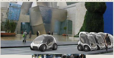
Launching in 2012. Price is estimated at 9.000€. It will be collapsible to facilitate parking, with a battery charging time of 12 minutes, 50 km/h of maximum speed and 120 km of range.
