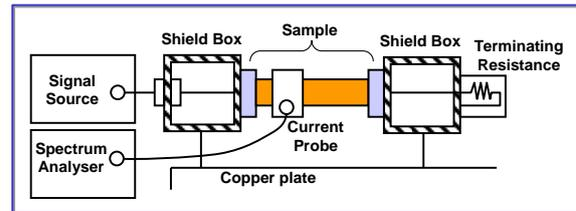
\*System configuration and test method according CISPR 25
