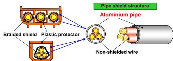
Figure 5: The concept of pipe shield wiring harness
