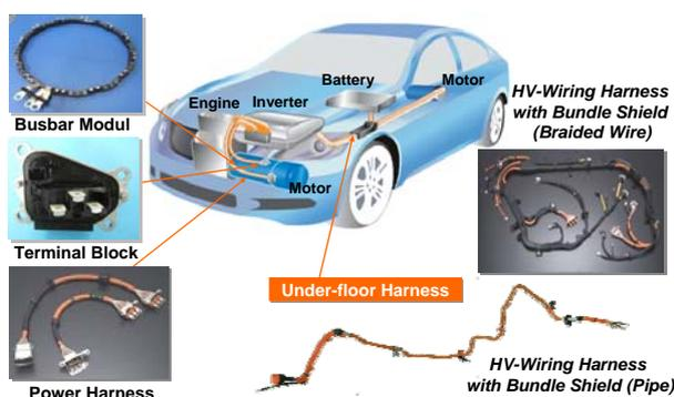
Figure 2: High-voltage technologies within the Sumitomo Electric Group and their location in a HEV
