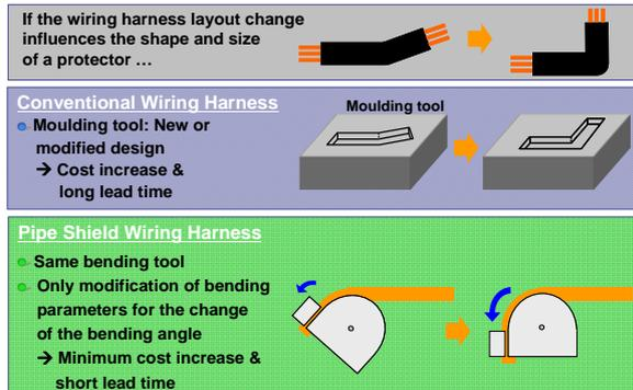
Figure 14: Simplification of wiring harness sheath design
