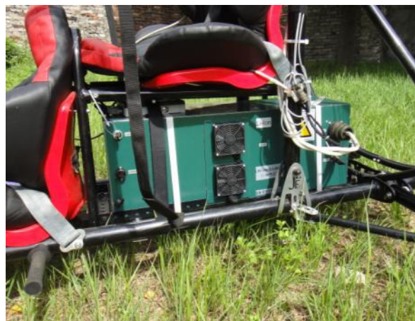
Figure5: The battery pack mounted in paraglider under the seat of the passenger
