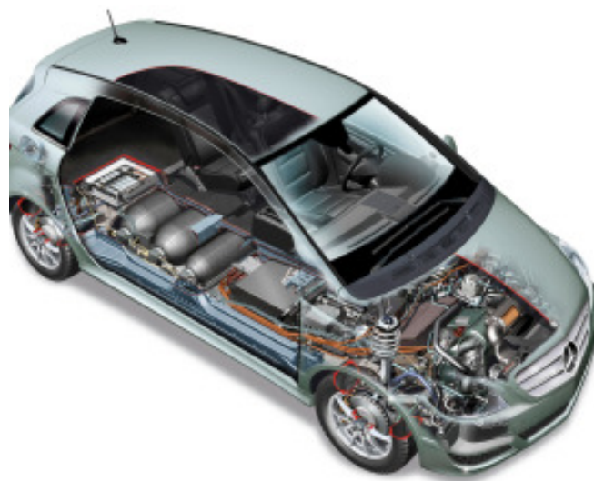
Figure 4. Packaging of the F-Cell B-Class, showing from left to right: high voltage battery, hydrogen tank, fuel cell stack, hydrogen module and in the front the air the air system placed above the electric drivetrain in the engine compartment.
