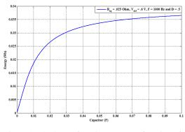
Figure 9: SSC transferred energy as a function of capacitor value.
