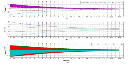
Figure 6: Switched capacitor simulation results. a) Cells and capacitor C<sub>1</sub> (between cells 1&2) voltages, b) Cells SoC, c) Cells currents
