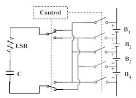
Figure 4: Single switched capacitor (SSC). [2]
