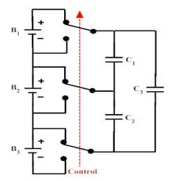
Figure 3: Double-Tiered switched capacitor (DTSC). [2]
