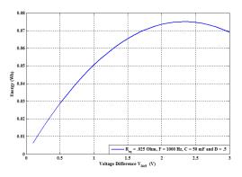
Figure 11: SSC transferred energy as a function of Voltage difference.
