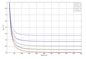
Figure 14: SSC equivalent resistor  $R_{equ}$  as a function the switching frequency F and the duty cycle D.
