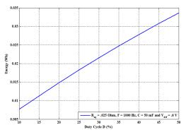
Figure 13: SSC transferred energy as a function of duty cycle D.
