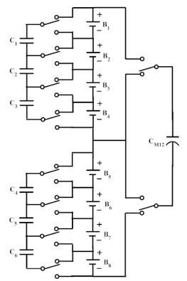
Figure 5: Modularized switched capacitor (MSC). [2]
