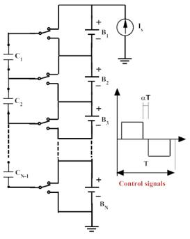
Figure 2: Switched capacitor (SC). [2]
