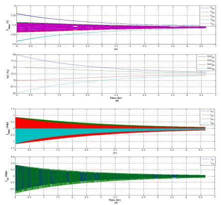
Figure 7: Double-Tiered switched capacitor simulation results. a) Cells and capacitor C<sub>2</sub> (between cells 2&3) voltages, b) Cells SoC, c) Cells currents and d) Capacitors C<sub>1</sub> and C<sub>4</sub> (second tier capacitor) currents
