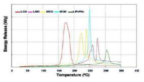
Figure 6: Energy released at various temperatures for the different cathode materials
