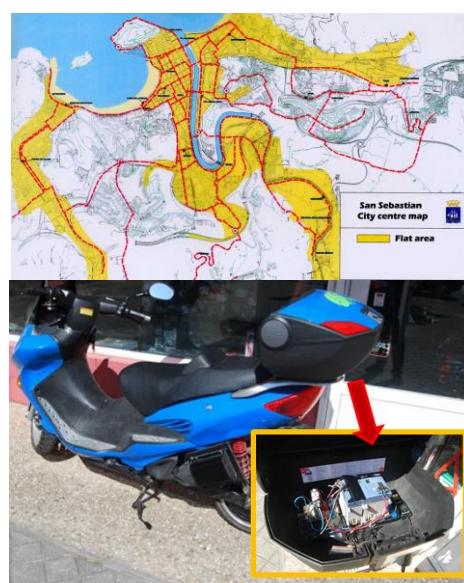
Figure 2: San Sebastian city centre map and logging hardware installed in an electric scooter.
