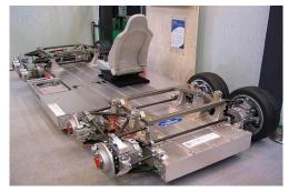
Figure 3: Eliica 8WD Internal structure
