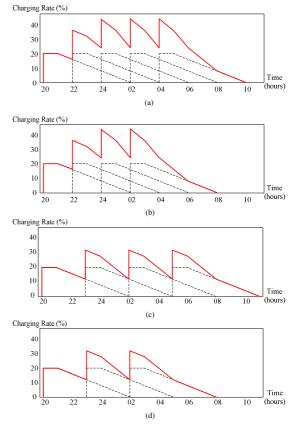
Figure 5: Simulated charging characteristics for different combination of groups/separating hours: (a) 5/2; (b) 4/2; (c) 4/3; and (d) 3/3
