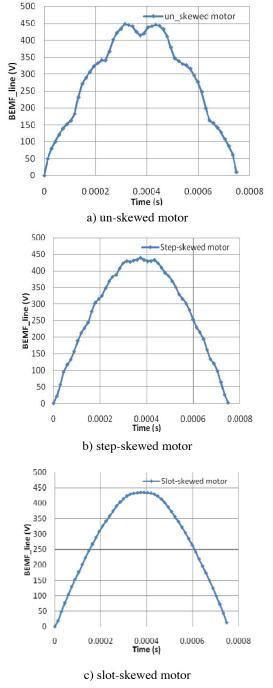
Fig. 3 Simulation no-load Back EMF
