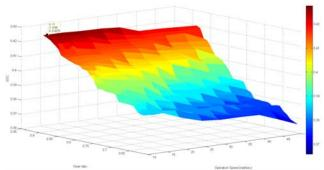
Figure 13: Optimization of parameters map for fixed inertia flywheel
