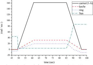
Figure 12: ECE cycle for each component in 45~100 sec
