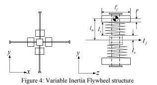
To adjust or to change the inertia of the flywheel, can be in many different ways. It will certainly affect the ability of the flywheel in storing or releasing kinetic energy. In this case, the inertia of variable inertia
