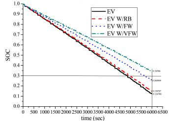
Figure 14: SOC<sub>remained</sub> of vehicles using NewYork bus cycle
