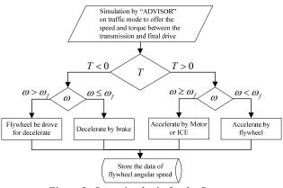
Figure 2: Operating logic for the System
