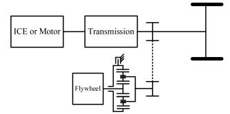
Figure 1: The Hybrid Power System Structure
