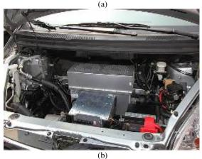
Figure 5: Propulsion Driving System in engine room
