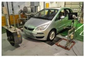
Figure 10: Emission & Fuel Economy Testing Lab to LDV.
