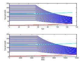
Figure 6: The relationship map of the motor T-N curve and the running resistance
