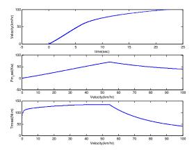
Figure 7: The 0-100km/hr acceleration time, motor P-N and T-N
