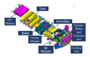
Figure 2: Drive Train B-Class F-CELL
