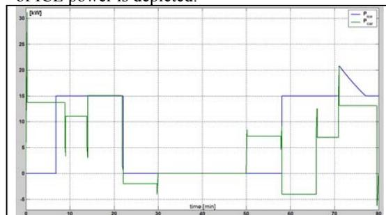
Figure 5. Time dependence of vehicle power demands during driving cycle. Blue line – ICE power, green line- power on driving wheels needed for vehicle movement
