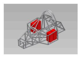
Figure 10: Placement of the batteries
