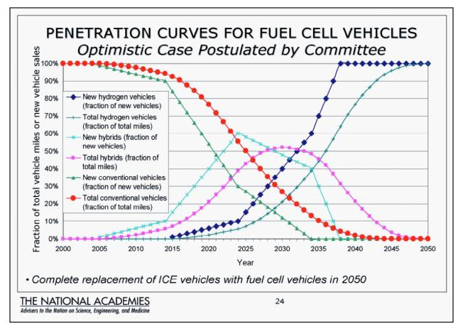
Figure 1: Market penetrations scenarios for hybrid and fuel cell powered vehicles
