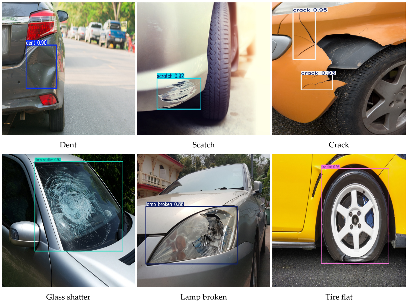
Figure 8. Qualitative detection results of the proposed method on representative vehicle damage images.
