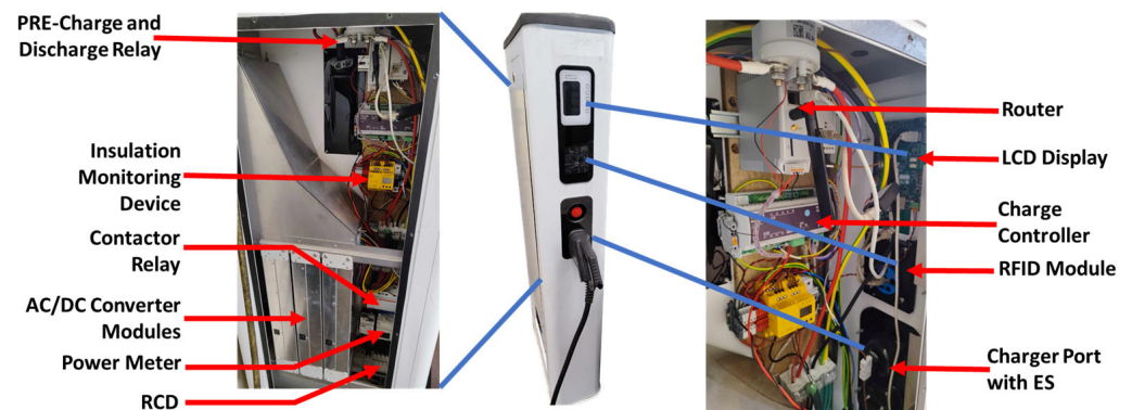
Figure 14. Hardware prototype of 45 kW rated modular DC charging container.
