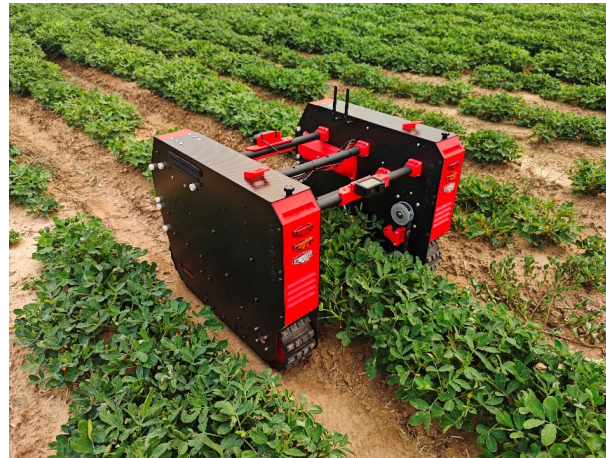
Figure 9. Field testing of the rubber-tracked robot chassis.
