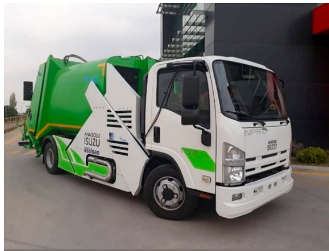
Figure 2. Series hybrid refuse truck used for real-world data collection and controller prototyping.
