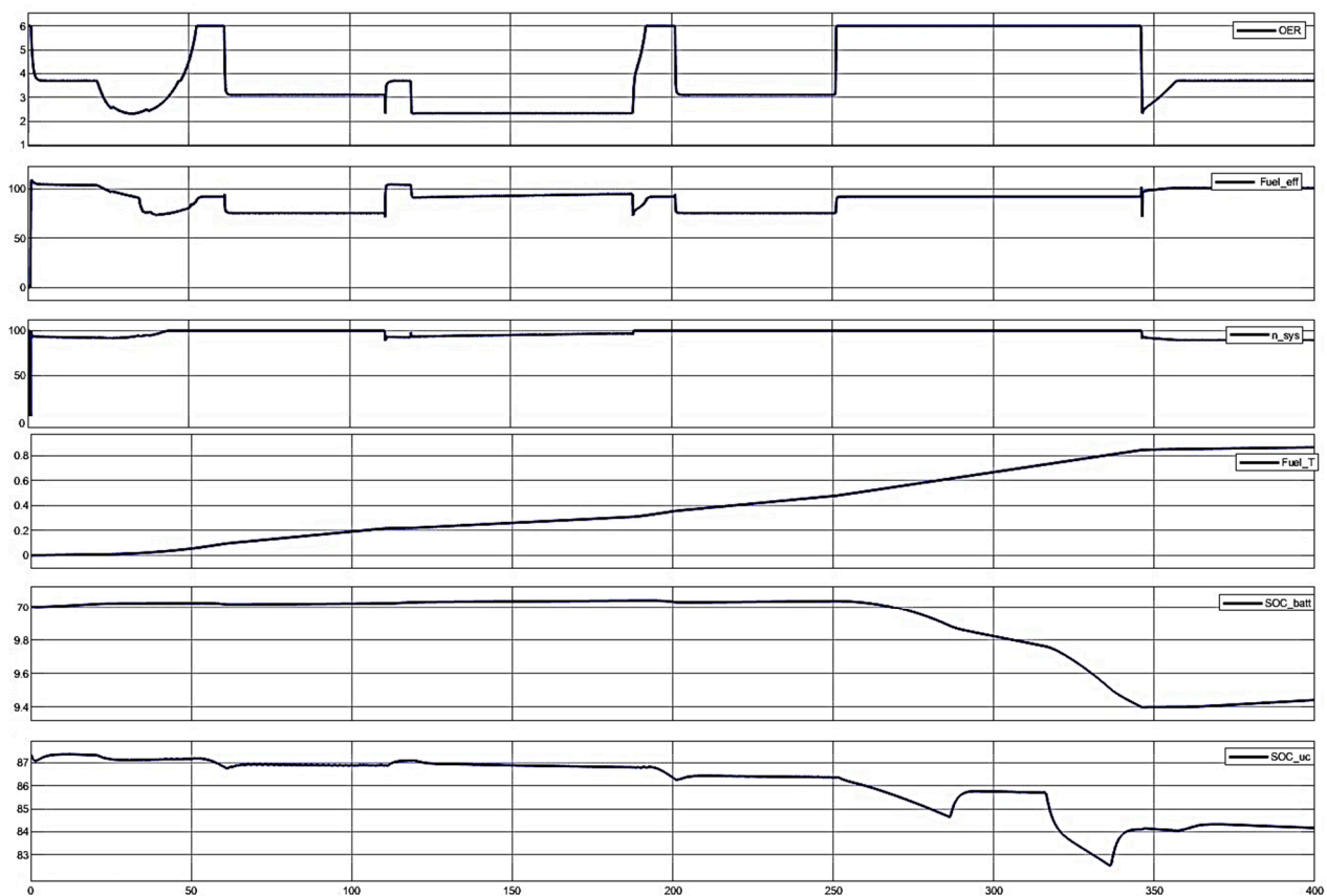
Figure 8. Profiles of the performance indicators used (oxygen excess ratio (OER), fuel efficiency ( Fuel_{eff} ), energy efficiency ( \eta_{eff} ), total fuel consumption ( Fuel_T ), and state of charge (SOC) of batteries and ultracapacitors) in a 30 kW fuel cell configuration.
