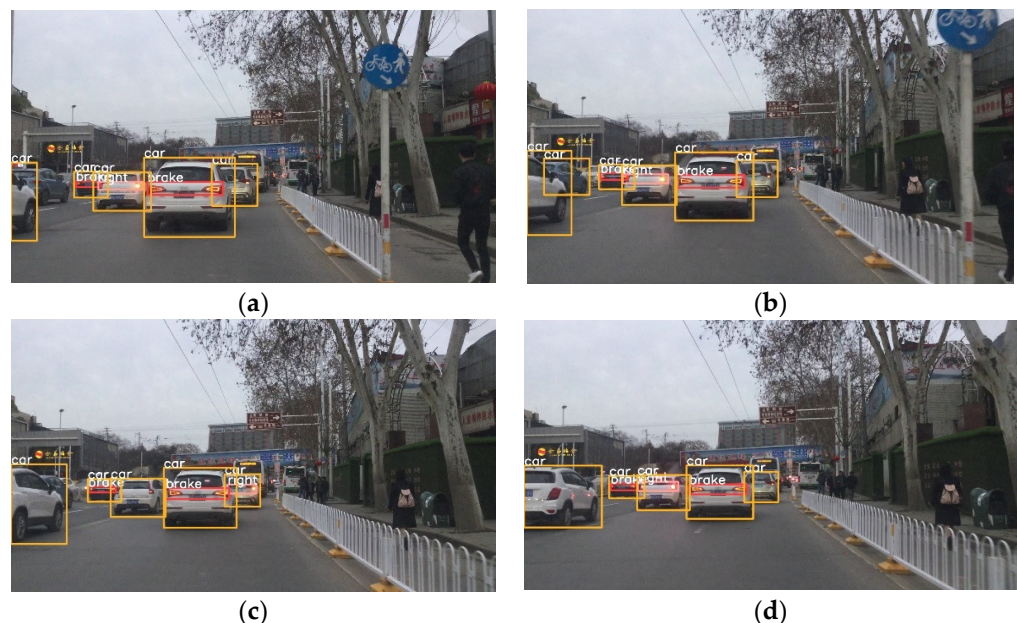
Figure 17. Consecutive figure detection results. (a) is the first frame; (b) is the second frame; (c) is the third frame; and (d) is the forth frame, orange boxes are detected vehicle taillights.
