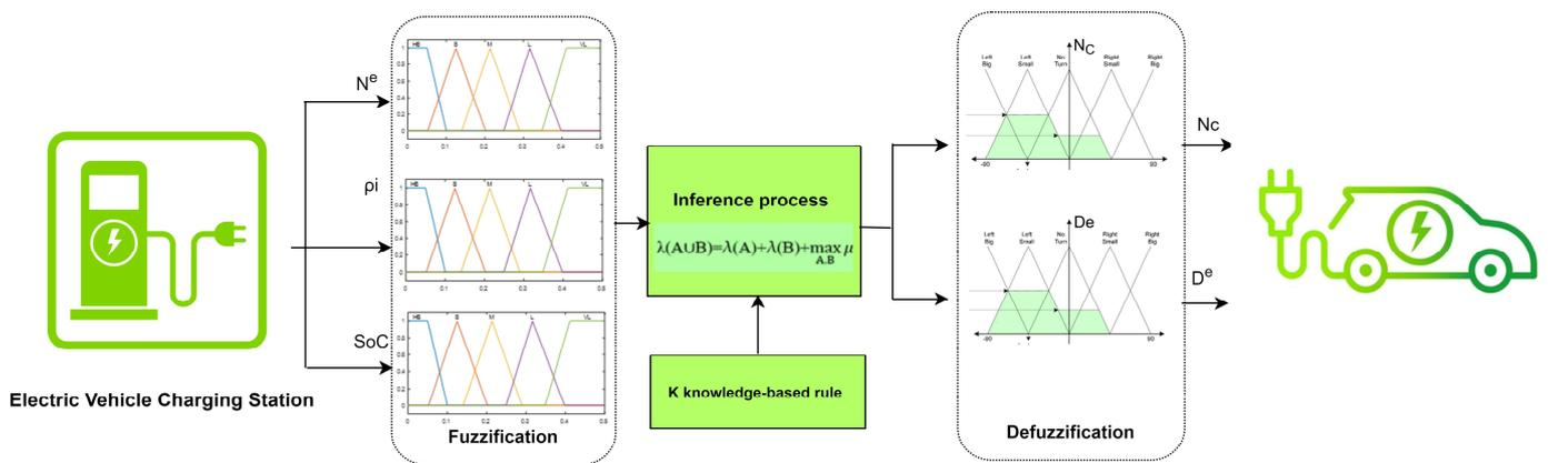
Figure 2. Block diagram of K-additive FLC for the electric charging station.
