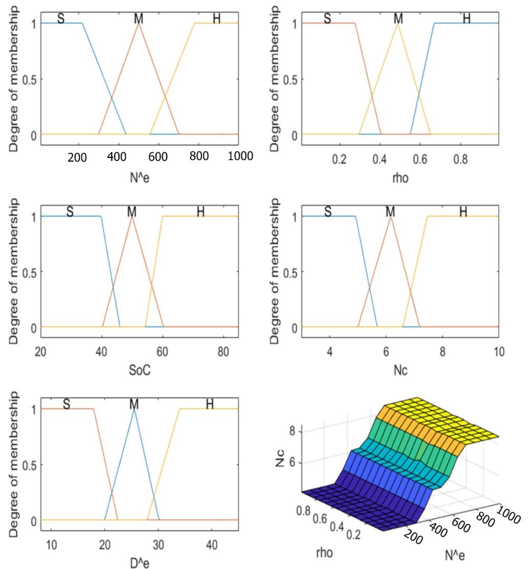
**Figure 3.** Fuzzy membership functions of variables and fuzzy surface. S stands for small range, M for medium range and H is for high range.
