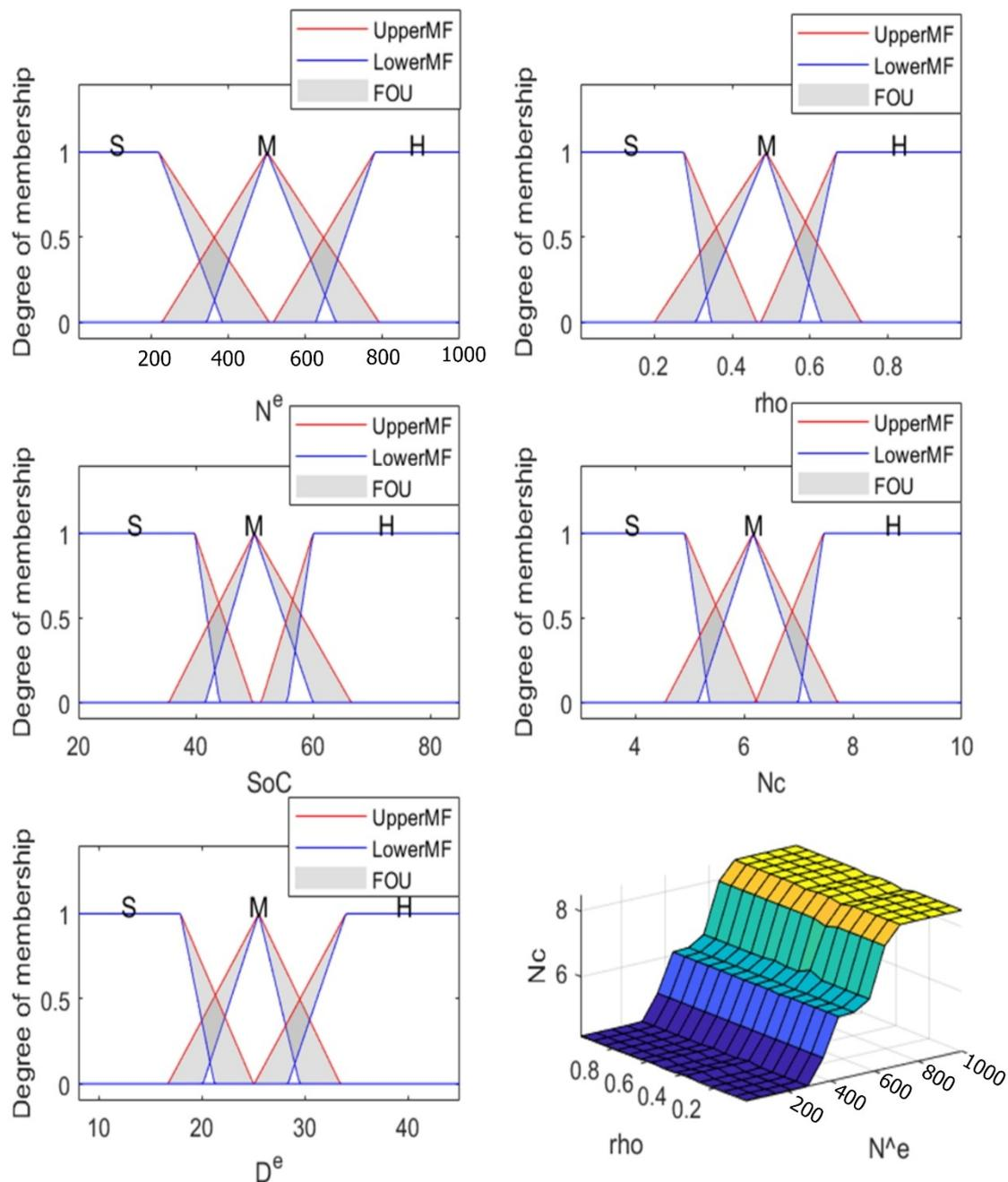
**Figure 4.** Type 2 fuzzy membership functions of variables and fuzzy surface. S stands for small range, M for medium range and H is for high range.
