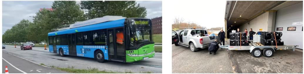
**Figure 8.** (Left): An electric bus and a passenger car drawing power from the ERS demonstrator simultaneously. (Right): The trailer designed to draw 300 kW.
