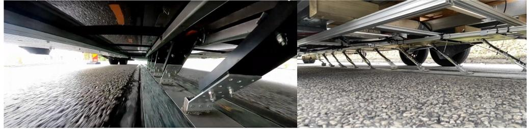
**Figure 5.** Two different types of pick-ups mounted on different vehicles providing contact between ASSE and vehicle.
