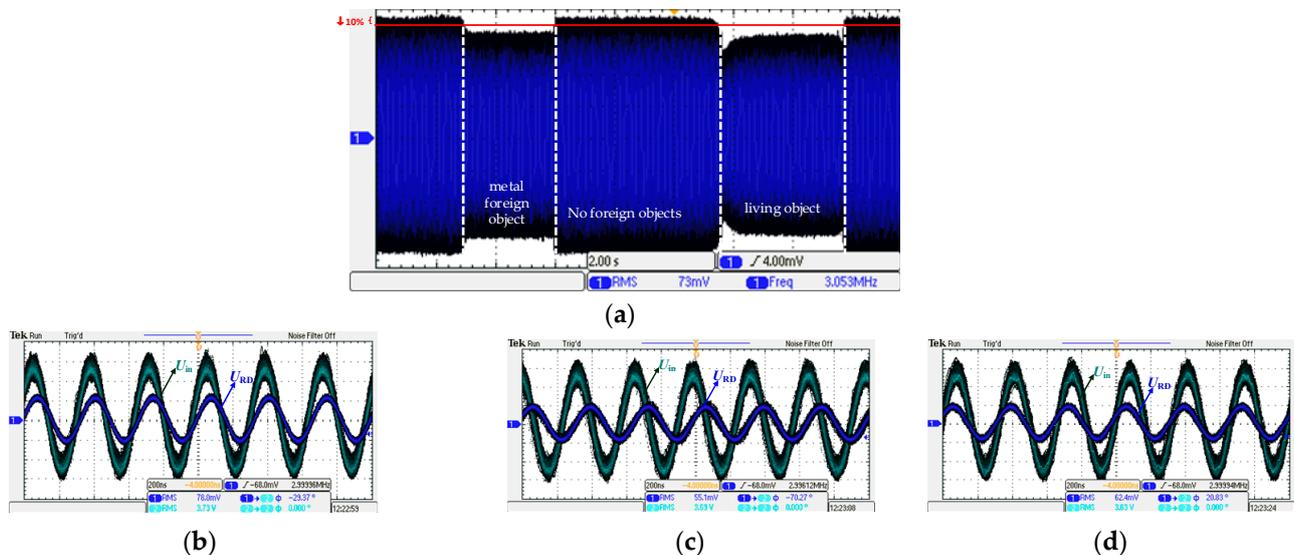
**Figure 17.** Waveforms of  $U_{in}$  and  $U_{RD}$  when metal and living organism foreign objects enter the detection region. (a) Metal and live foreign objects enter the detection area in sequence. (b) No foreign object. (c) Living organism foreign object (beef block). (d) Metal foreign object (metal screw).
