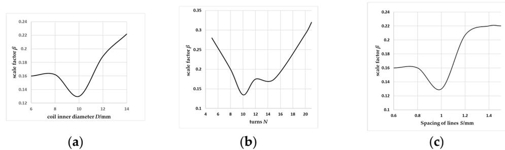
Figure 11. Curve of variation in scale factor  $\beta$  with coil diameter inside  $D$  and number of turns  $N$ , wire-to-wire spacing  $S$ . (a) The relationship between  $\beta$  and  $D$ . (b) The relationship between  $\beta$  and  $N$ . (c) The relationship between  $\beta$  and  $S$ .
