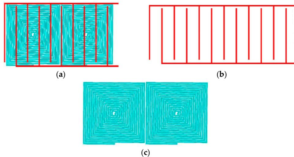
**Figure 12.** Array detection coil and comb capacitor combination mode. (a) Combined array detection coil. (b) Comb capacitor model. (c) Inverse series rectangular coil model.
