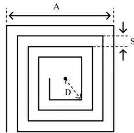
Figure 10. Square detection coil structure.
