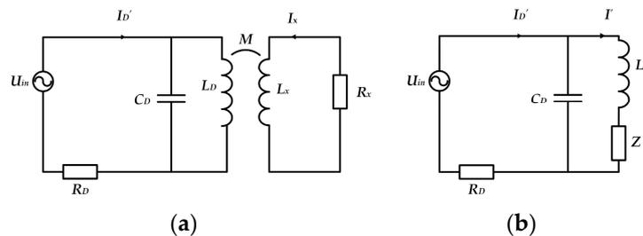
Figure 3. Equivalent circuit model of metal foreign object and detection coil. (a) Coupling model for metal foreign object and detection circuits. (b) Coupled model simplified circuit.
