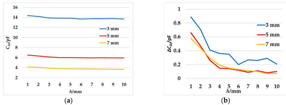
**Figure 6.** The variation in  $C_{Di}$  and  $\Delta C_{Di}$  with  $d$  and  $h$ . (a)  $C_{Di}$ . (b)  $\Delta C_{Di}$ .
