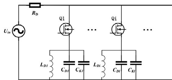
**Figure 13.** Equivalent circuit diagram of foreign object detection system.
