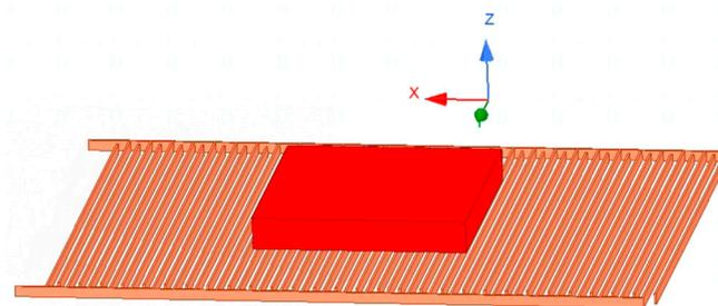
Figure 5. Finite element simulation model of comb capacitor (living foreign object).
