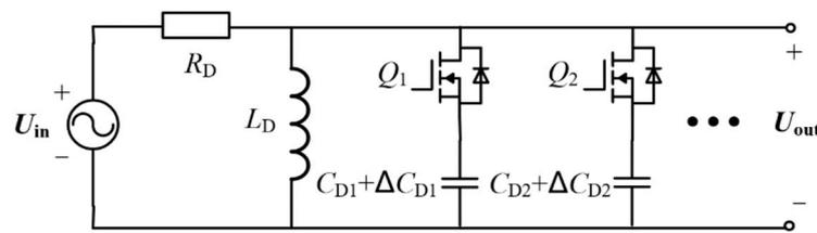
Figure 1. Live foreign object detection circuit.
