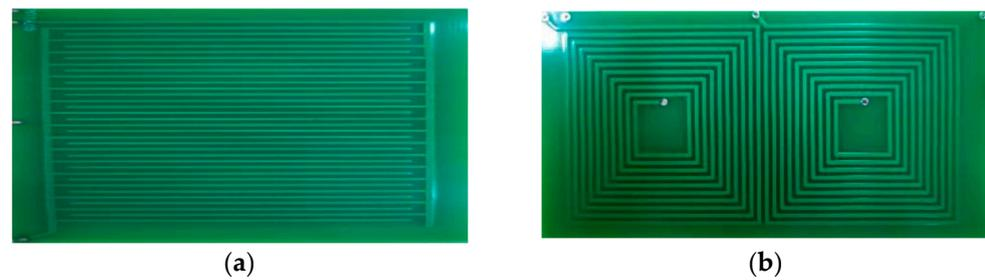
**Figure 15.** Combination of a detection coil and a comb capacitor: (a) front side (comb capacitor) and (b) reverse side (detection coil).
