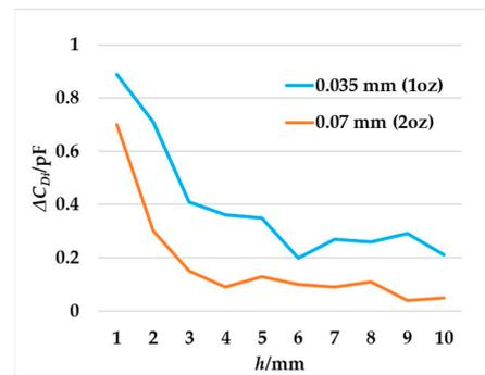
**Figure 8.** The variation in  $\Delta C_{Di}$  with  $h$  under different wire thicknesses.
