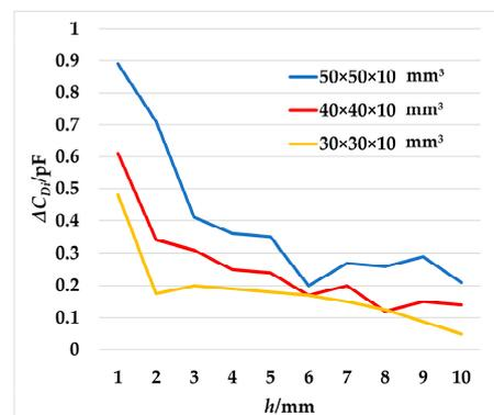
**Figure 7.** The variation in  $\Delta C_{Di}$  with  $h$  under different living foreign object sizes.
