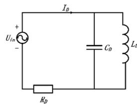
Figure 2. Foreign object detection circuit in the absence of foreign objects.
