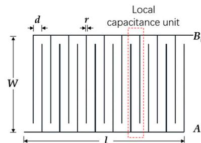
Figure 4. Basic structure of comb capacitor.
