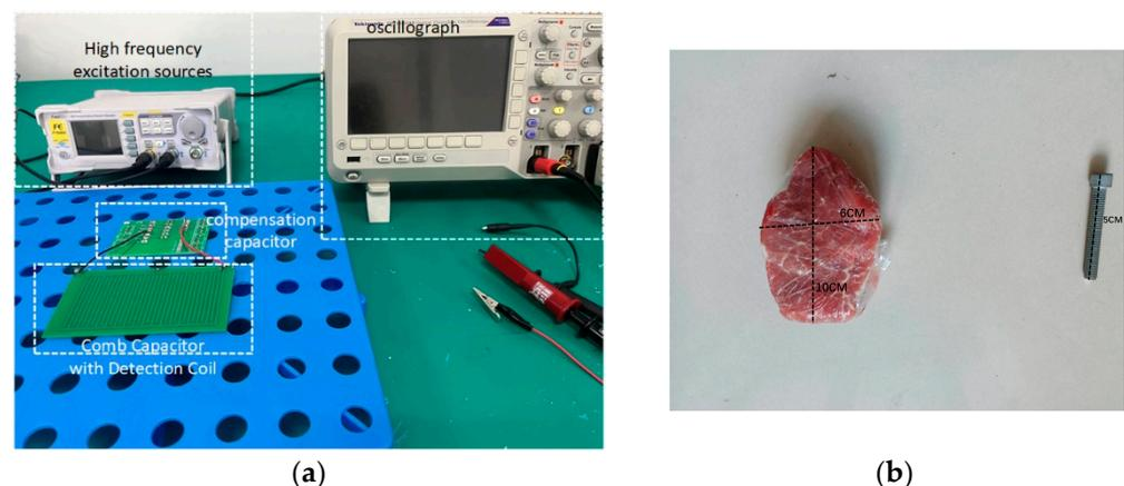
**Figure 16.** Experimental platform for foreign body detection. (a) Foreign object detection equipment. (b) Metal and living organism foreign objects.
