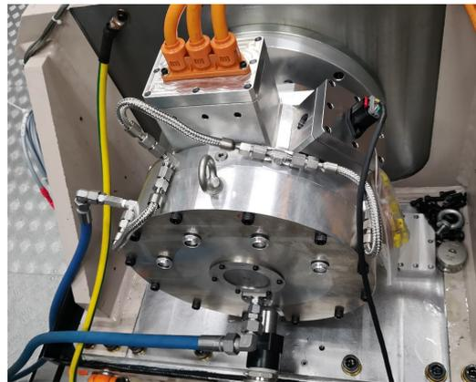
Figure 12. IWM prototype on the test bench.
