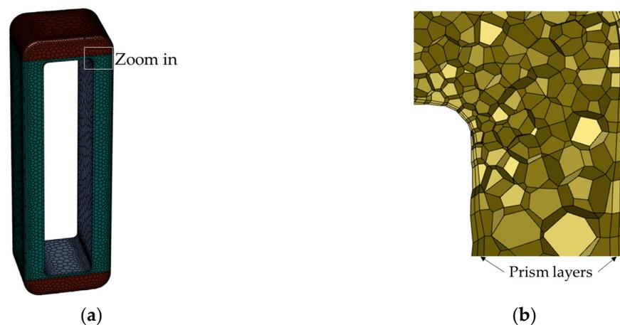
**Figure 6.** Mesh for solid: (a) one concentrated coil; (b) zoomed-in view of intensified prism layers.
