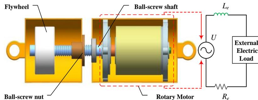
Figure 2. Ball-screw mechatronic inerter.
