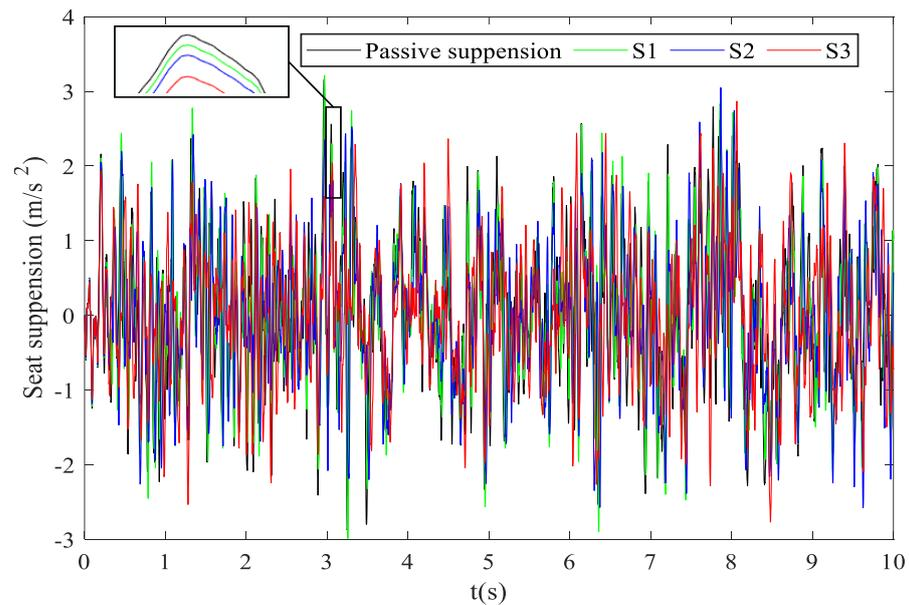
**Figure 6.** Comparison of the seat accelerations in the time domain.
