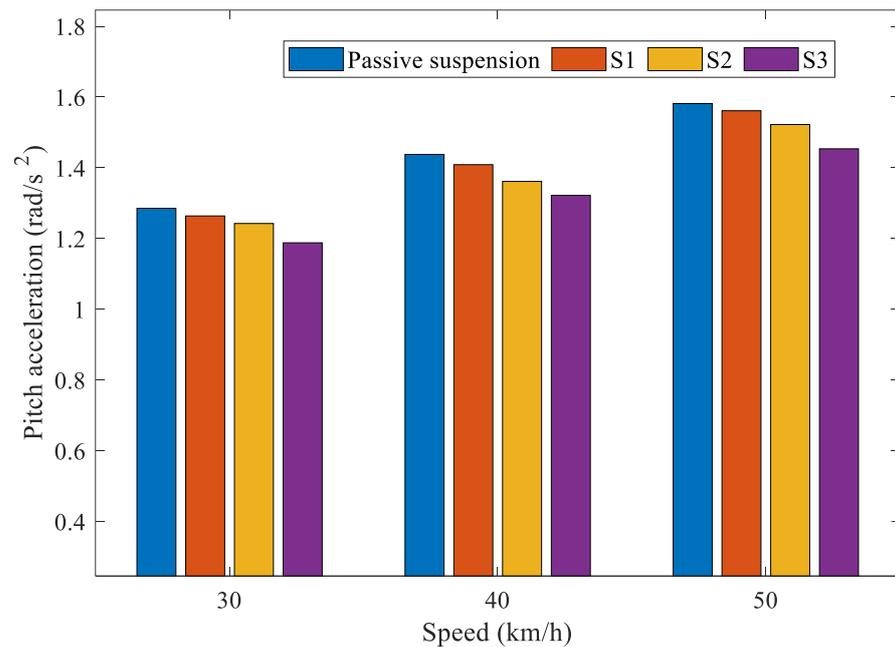
**Figure 9.** Comparison of the RMS of pitch acceleration under different speeds.
