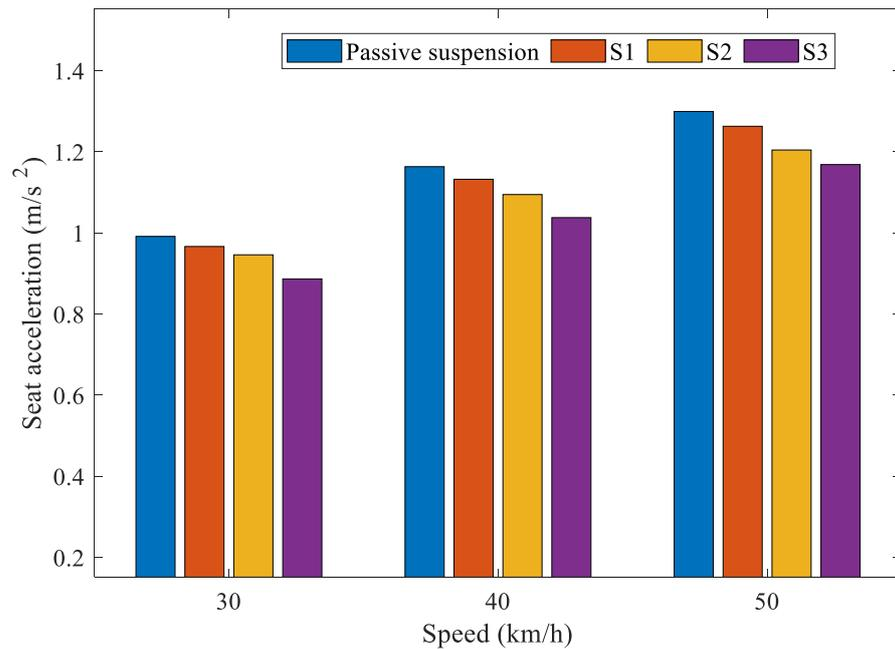
**Figure 8.** Comparison of the RMS of seat acceleration under different speeds.
