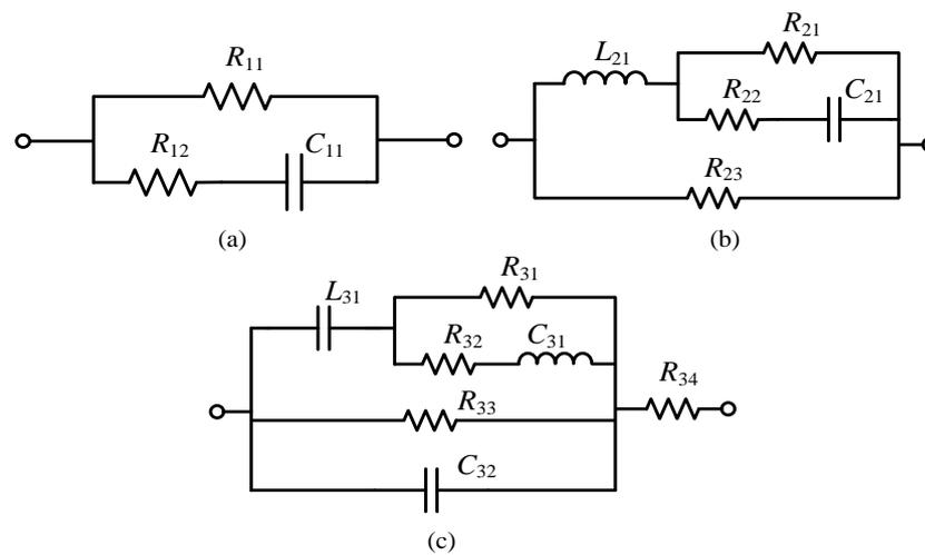
**Figure 5.** Electrical network. (a) Bivariate transfer function electrical network; (b) Biquadratic transfer function electrical network; (c) Bicubic transfer function electrical network.
