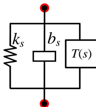
Figure 3. General layout of the seat suspension.
