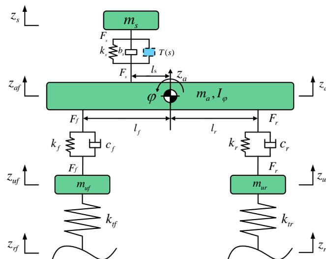
Figure 1. Seven-degree-of-freedom vehicle model.
