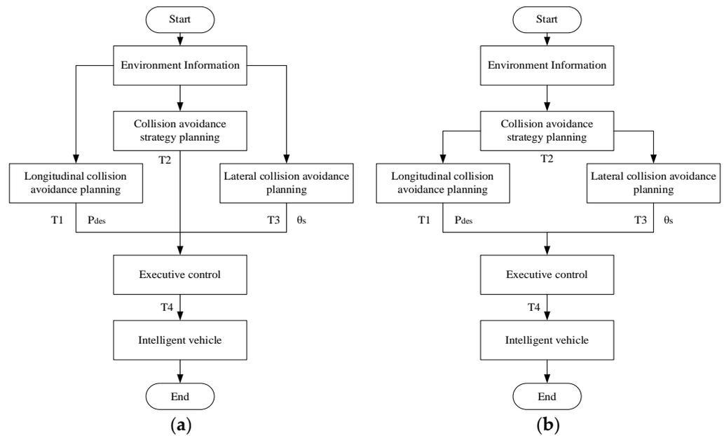
**Figure 6.** Active collision avoidance system control method: (a) Distributed coordinated control system; (b) Sequential control system.
