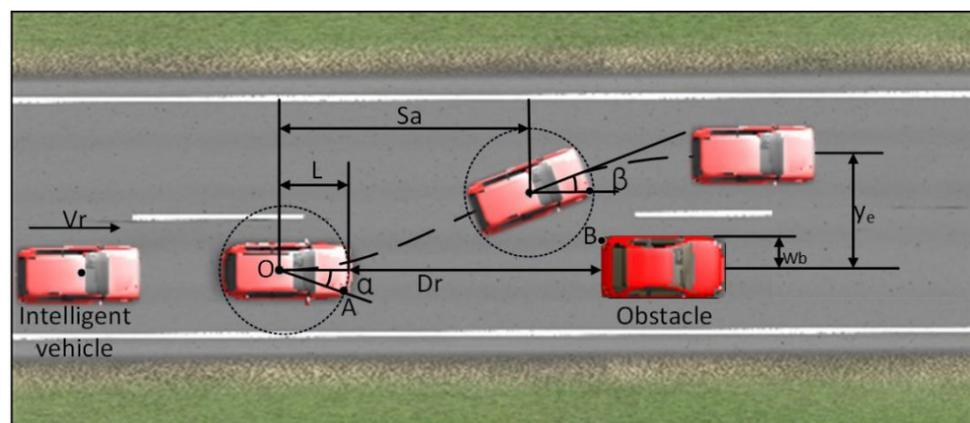
**Figure 2.** Intelligent vehicle lateral collision avoidance route.
