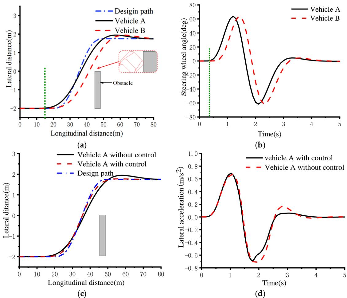
**Figure 9.** Simulation of lateral collision avoidance: (a) Lane-changing track; (b) Steering wheel angle; (c) Lane-changing track; (d) Lateral acceleration.
