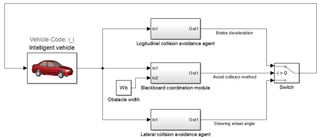
**Figure 7.** Distributed multi-agent collision avoidance system simulation.
