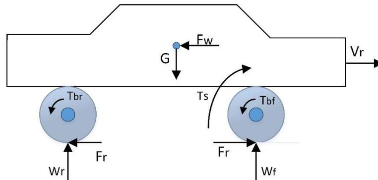
**Figure 1.** Diagram of vehicle force during braking.
