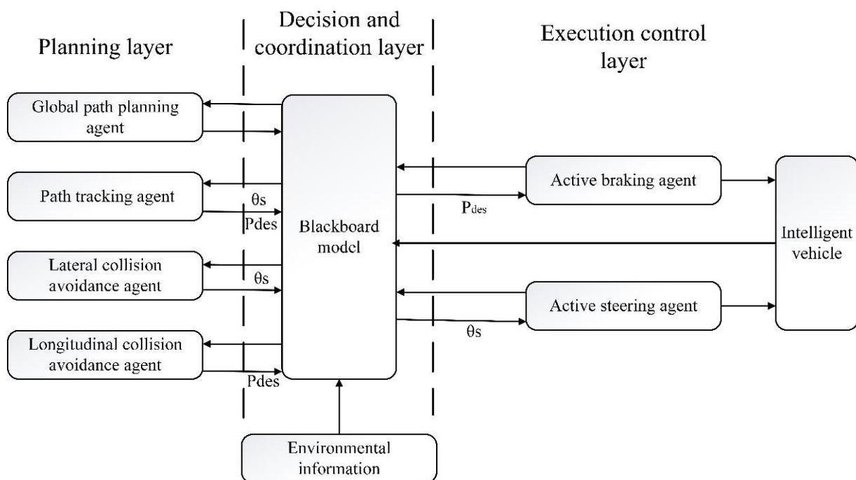
**Figure 4.** Multi-agent coordinated control system based on blackboard model.
