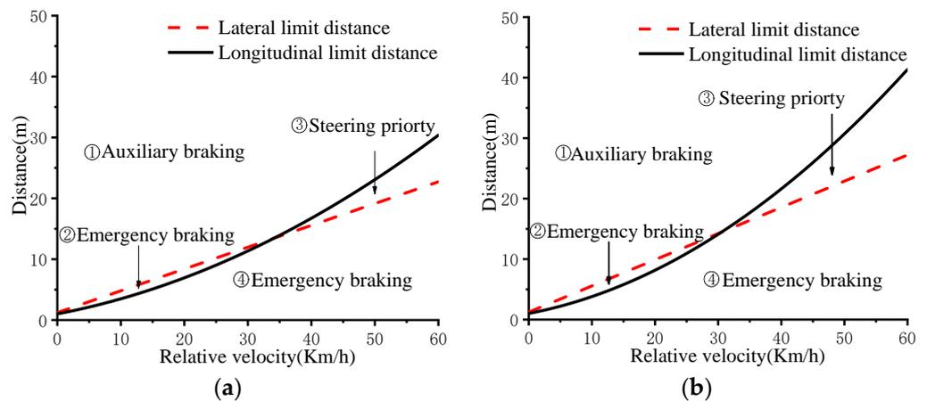
**Figure 5.** The choice of active collision avoidance during an emergency in different environments: (a) Dry asphalt pavement ( $\mu = 0.8$ ); (b) Wet asphalt pavement ( $\mu = 0.5$ ).
