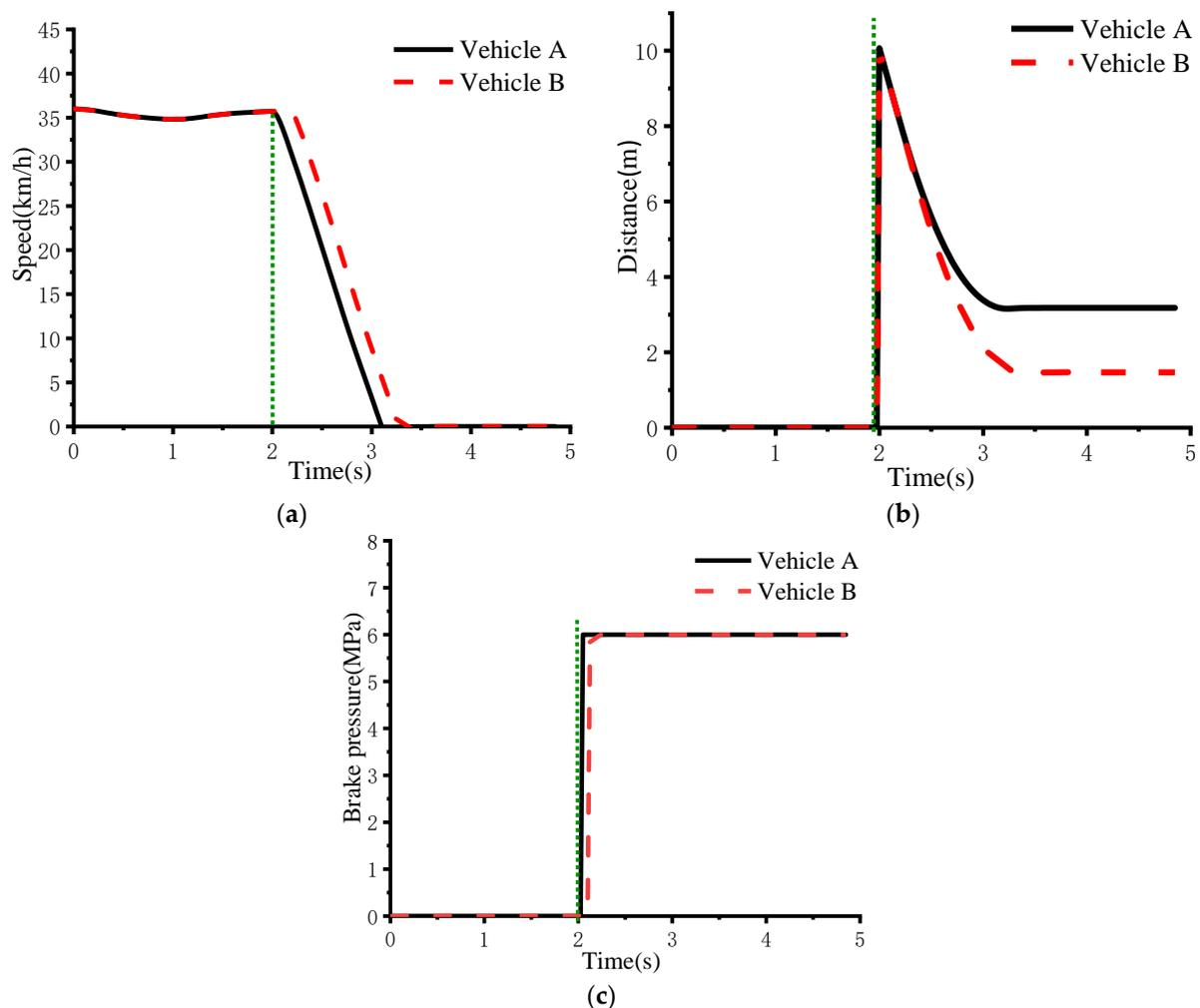
**Figure 8.** Simulation of longitudinal collision avoidance: (a) Vehicle speed; (b) Distance between vehicle and obstacle; (c) Brake pressure of the vehicles.
