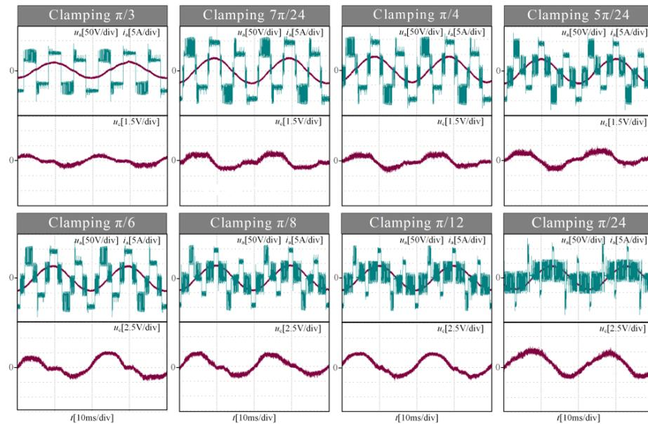
Figure 10. Experimental waveforms of eight clamping widths under the condition of  $m = 0.3$ .
