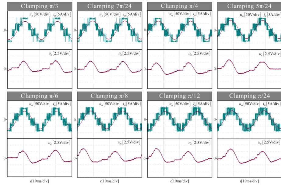
Figure 9. Experimental waveforms of eight clamping widths under the condition of  $m = 0.9$ .
