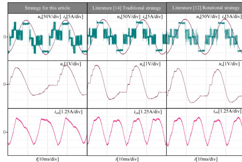
**Figure 14.** Comparison of experimental waveform under the condition of  $5 \Omega$  and  $10 \text{ mH}$ .
