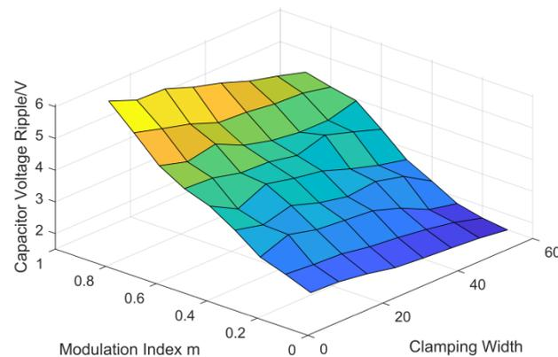
**Figure 12.** Capacitor voltage ripple.
