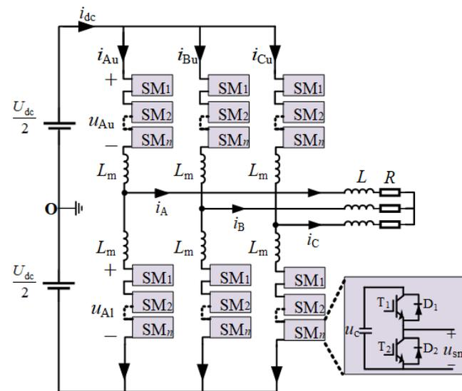
Figure 1. Topology of the three-phase modular multilevel converter (MMC).
