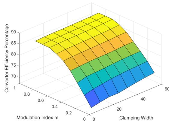
Figure 11. Converter working efficiency.
