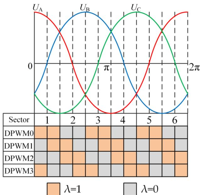
Figure 3. Clamping factor  $\lambda$  Schematic diagram of clamping interval.
