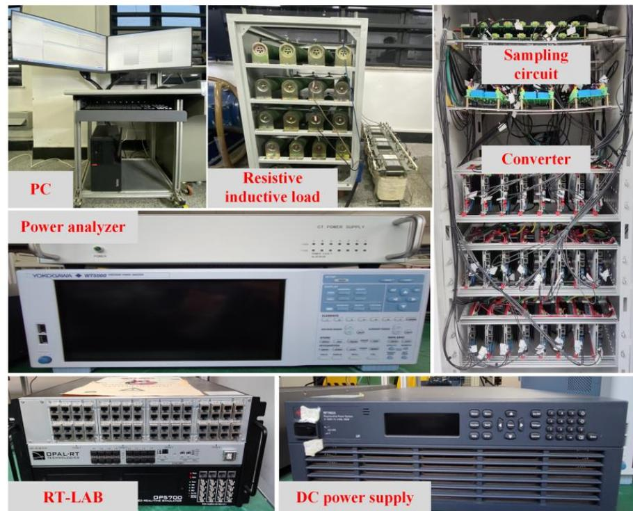
Figure 8. MMC experimental system diagram.
