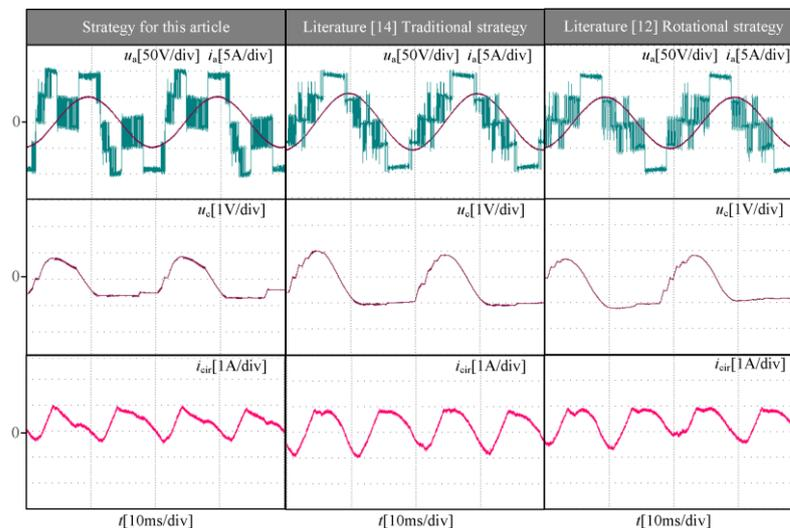
**Figure 15.** Comparison of experimental waveform under the condition of  $10 \Omega$  and  $30 \text{ mH}$ .
