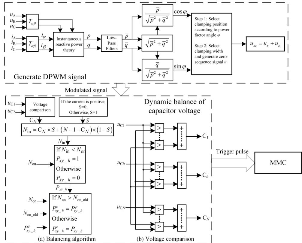
Figure 4. System control block diagram.
