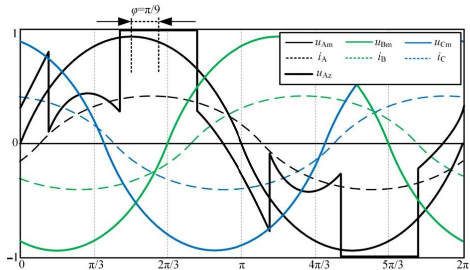
**Figure 7.** Example of discontinuous modulation strategy for variable load power factor.
