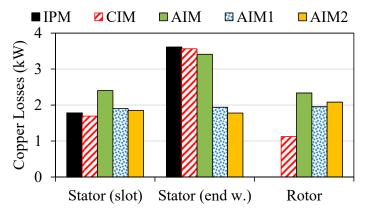
**Figure 13.** Comparison of copper losses including stator in-slot winding, stator end-windings, and rotor bars.
