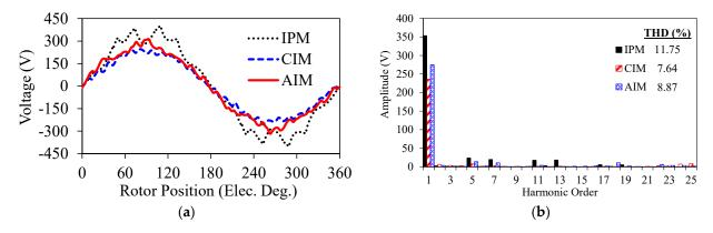
**Figure 3.** Comparison of back-EMF waveforms and their harmonic spectra. (a) Line Back-EMF and induced voltage waveforms. (b) Harmonic spectra of the back-EMF and induced voltage.
