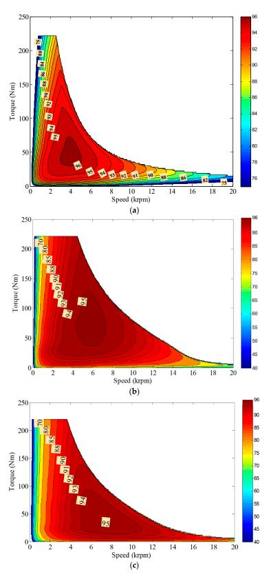
**Figure 7.** Comparison of the efficiency maps of the considered machines. (a) IPM machine. (b) CIM. (c) AIM.
