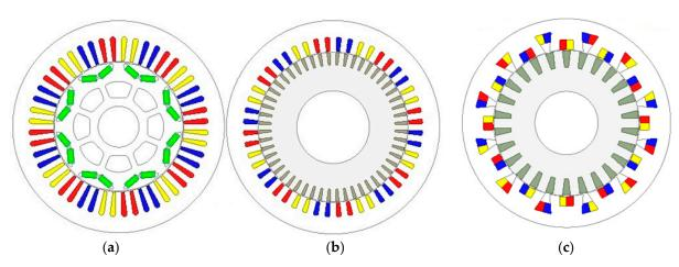
Figure 1. Two-dimensional views of the compared machines: (a) IPM (48S/16M/8P). (b) CIM (48S/52R/8P). (c) AIM (24S/26R/8P).
