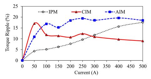
Figure 10. Comparison of torque ripple percentage for different electric loadings.
