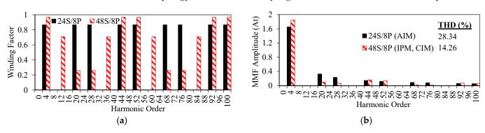
**Figure 2.** Comparison of winding factors and MMF harmonics of the considered machines. (a) Winding factors of harmonics. (b) MMF harmonics spectra for 1-turn and 1-ampere.
