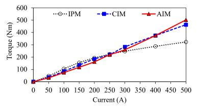
Figure 9. Comparison of torque production capabilities.
