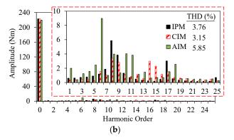
**Figure 5.** Comparison of the torque waveforms and their spectra. (a) Electromagnetic torque waveforms. (b) Harmonic spectra of torque.
