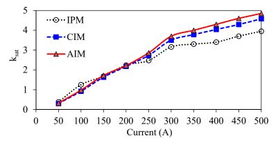
Figure 12. Variation of saturation factor with respect to electric loading.
