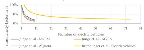
**Figure 2.** SFs reported in the literature by Junge et al. [12] (three scenarios) and by Bründlinger et al. [18] for electric vehicle charging. An SF of 100% was equivalent to all observed vehicles charging simultaneously at one moment in time. For a description of the individual scenarios, please refer to the linked studies.
