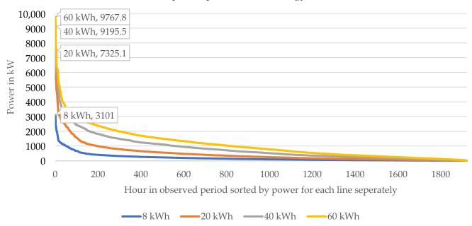
**Figure 12.** Sorted summed connector power when employing the price optimization strategy. For example, if during each charging process 40 kWh should be charged, during ~1400 h of the observed 1921 h, the chargers consumed 1000 kW or less.
