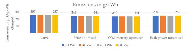
**Figure 17.** CO<sub>2</sub> intensity of the electricity charged from the grid using assumed energy recharged per charge event and charging strategies.
