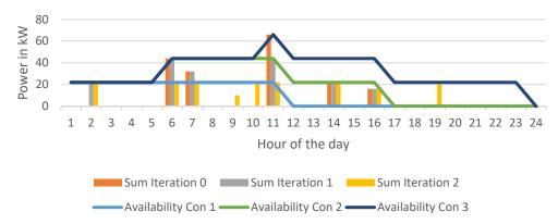
**Figure 8.** Example of the peak power reduction algorithm. Legend entries starting with "Sum" show the sum of the power demand of the three observed connecters for each iteration. Labels starting with "Availability" show the difference between the sum of the charging power of all connected vehicles and the already scheduled recharges at that instance.
