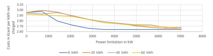
**Figure 16.** Costs in EURcent per kWh net recharged energy as a function of the global power limit for the power limits defined in Section 3.2. The left end is the same as "peak minimisation" and the right end is almost identical to the "price optimised" in Figure 15 as a little peak minimisation is required with a power limit of over 7040 kW.
