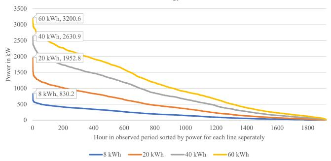
**Figure 11.** Sorted summed connector power when employing the naive strategy. For example, if during each charging process 40 kWh is to be charged, during ~800 h of the observed 1921 h, the chargers consumed 500 kW or less.
