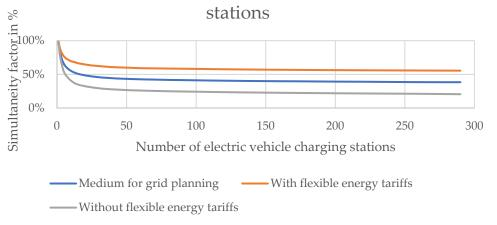
**Figure 3.** SFs reported in the literature [16] for electric vehicle charging stations. An SF of 100% is equivalent to all observed charging stations having a vehicle charging at full power at one moment in time.
