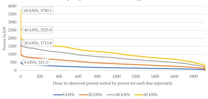
**Figure 14.** Sorted summed connector power when employing the peak minimization strategy. For example, if during each charging process 40 kWh should be charged, during ~400 h of the observed 1921 h, the chargers consumed 500 kW or less.
