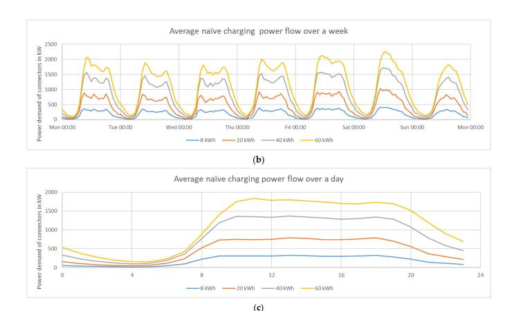
**Figure 9.** Power demand using the naive charging strategy for the 1562 connectors with a total power of ~34 MW observed in this study: (a) the power flow over the entire simulated timeframe; (b) the average of (a) over a week; (c) the average of (a) over a day. The plot is structurally very similar to Figure 5.
