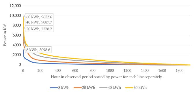
**Figure 13.** Sorted summed connector power when employing the  $CO_2$  optimisation strategy. For example, if during each charging process 40 kWh should be charged, during ~200 h of the observed 1921 h, the chargers feed in power at a rating of 4000 kW or more.
