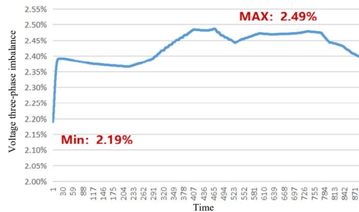
Figure 6. Three-phase voltage imbalance in the distribution network.
