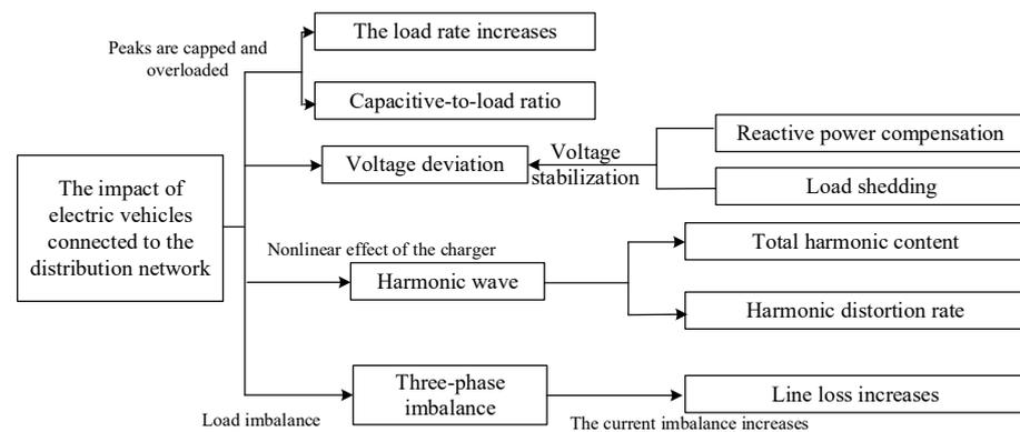
**Figure 3.** The impact of electric vehicle charging loads on various indicators of the distribution network.
