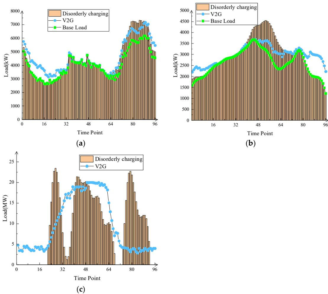
**Figure 7.** Load curves of disordered charging mode and V2G mode in various regions. (a) Load curves in residential areas; (b) the load curves of the business district; (c) charging station load curves.
