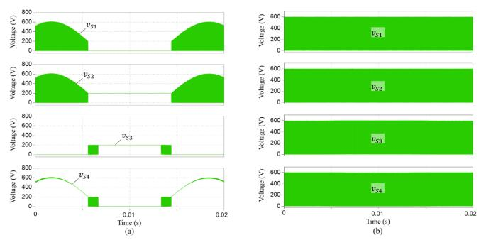
Figure 12. Voltage across the switch devices in a phase module. (a) BBI and (b) B-VSI.
