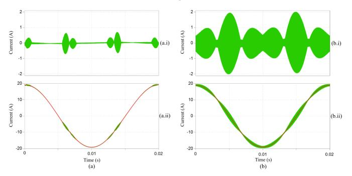
**Figure 7.** Simulated ripple characteristics of the output current of the (**a**) BBI and (**b**) B-VSI. (**a.i,b.i**) Ripple component of the output current and (**a.ii,b.ii**) instantaneous (green) and averaged (red) waveform of the output current.
