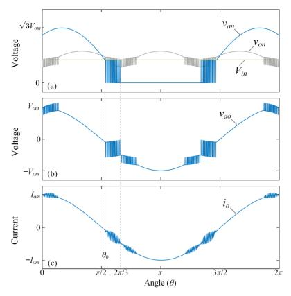
**Figure 5.** The characteristic waveforms of (**a**) the module output voltage  $v_{an}$ , load neutral voltage  $v_{on}$ , (**b**) the phase voltage  $v_{ao}$ , and (**c**) current  $i_a$  of the load.
