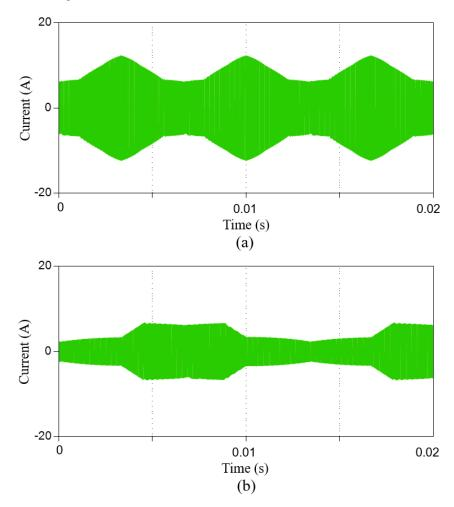
**Figure 11.** Simulated waveforms of the ripple of the three summed input inductor currents (**a**) without and (**b**) with the phase swapping interleaving method.
