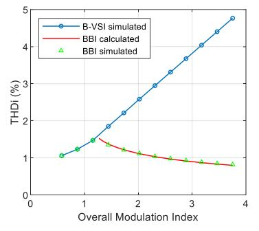
Figure 8. THD of the output current of the two topologies at different overall modulation indexes.
