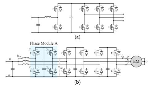
**Figure 1.** Circuit topology of (**a**) B-VSI: voltage source inverter with a preceding booster stage and (**b**) BBI: boost-buck inverter.
