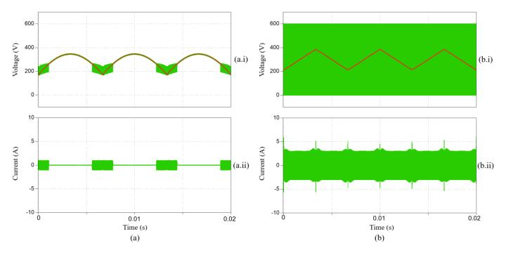
**Figure 9.** Simulated output CM voltage and current of the (**a**) BBI and (**b**) B-VSI. (**a.i**,**b.i**) Instantaneous (green) and averaged (red) waveform of the CM voltage and (**a.ii**,**b.ii**) CM current.
