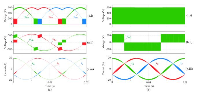
**Figure 6.** Simulated output voltage and current waveforms of the (**a**) BBI and (**b**) B-VSI. (**a.i**,**b.i**) Phase voltages, (**a.ii**,**b.ii**) phase-to-phase voltages, and (**a.iii**,**b.iii**) output currents.
