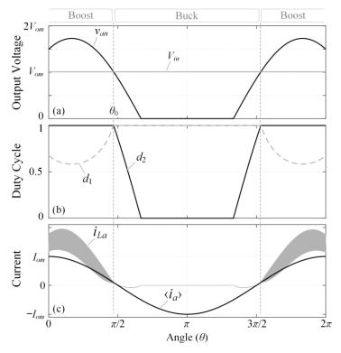
**Figure 3.** The characteristic waveforms of phase module A of the boost-buck inverter. (**a**) The input voltage  $V_{in}$ , reference output voltage  $v_{an}$ , (**b**) duty cycle  $d_1$  for the boost switch leg, duty cycle  $d_2$  for the buck switch leg, (**c**) input current  $i_{La}$ , and average output current  $i_a$  are shown.
