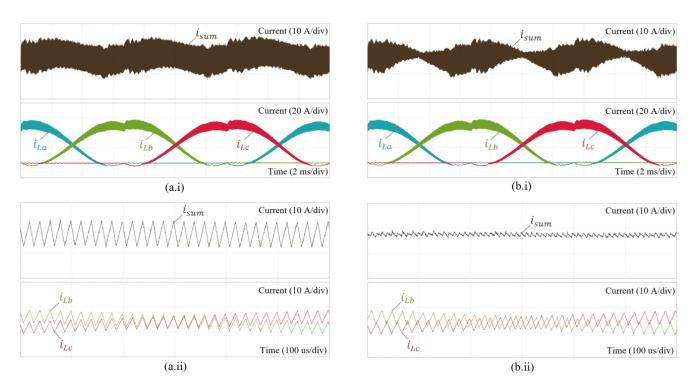
**Figure 16.** Measured waveforms of the input inductor currents ( $i_{La}$ ,  $i_{Lb}$ ,  $i_{Lc}$ ,  $i_{sum} = i_{La} + i_{Lb} + i_{Lc}$ ) of the BBI. (**a**) Without interleaving. (**b**) With interleaving. (**a.i**,**b.i**) Waveforms over a fundamental cycle. (**a.ii**,**b.ii**) Zoomed-in detail of the waveforms.
