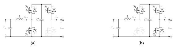
Figure 2. The two modes of a phase module of the BBI: (a) boost mode and (b) buck mode.
