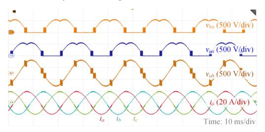
**Figure 13.** Experimental waveforms of the output phase voltages ( $v_{an}$  and  $v_{bn}$ ), phase-to-phase voltage  $v_{ab}$ , and three-phase currents ( $i_a$ ,  $i_b$ , and  $i_c$ ) of the BBI.
