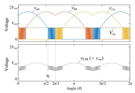
Figure 4. The characteristic waveforms of three-phase output voltages and the CM voltage.
