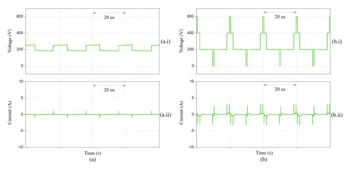
**Figure 10.** Zoomed-in detail of the CM voltage and current waveforms. (**a**) BBI and (**b**) B-VSI. (**a.i**,**b.i**) CM voltage and (**a.ii**,**b.ii**) CM current.
