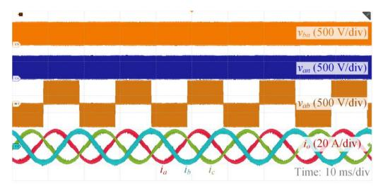
**Figure 14.** Experimental waveforms of the output phase voltages ( $v_{an}$  and  $v_{bn}$ ), phase-to-phase voltage  $v_{ah}$ , and three-phase currents ( $i_a$ ,  $i_h$ , and  $i_c$ ) of the B-VSI.
