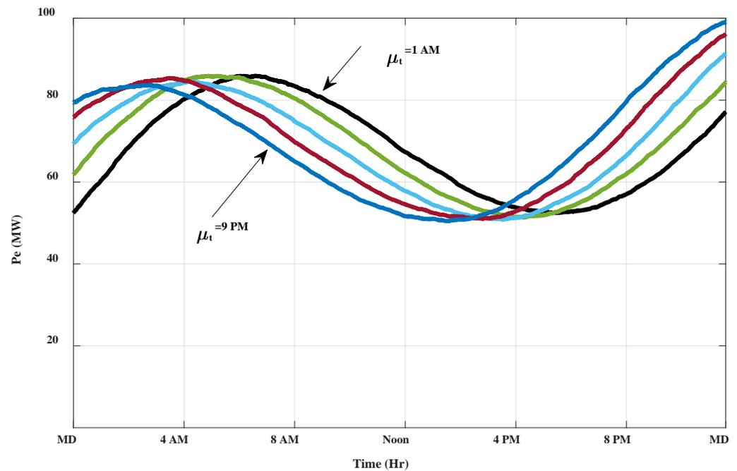
**Figure 15.** Final set of the load curve of EVs demand at different mean times.
