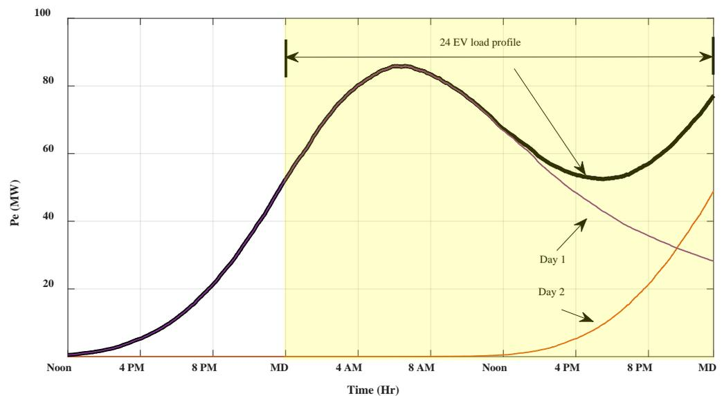
Figure 14. Derivation of the 24 h demand profile of a daily 100 thousand 100 vehicles distributions.
