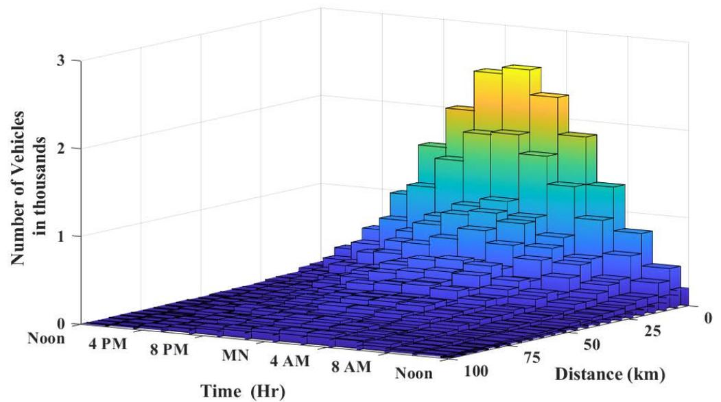
Figure 12. Distribution of both arrival time and travelled distance for 100 k vehicles.
