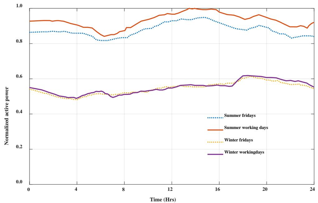
Figure 5. Typical daily load curves of the Saudi electrical power system of the year 2019.
