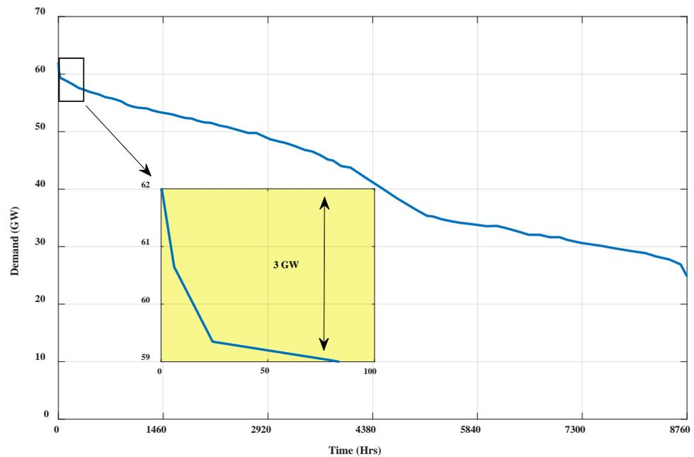
Figure 6. Typical Load duration curve of the national Saudi power system 2019.
