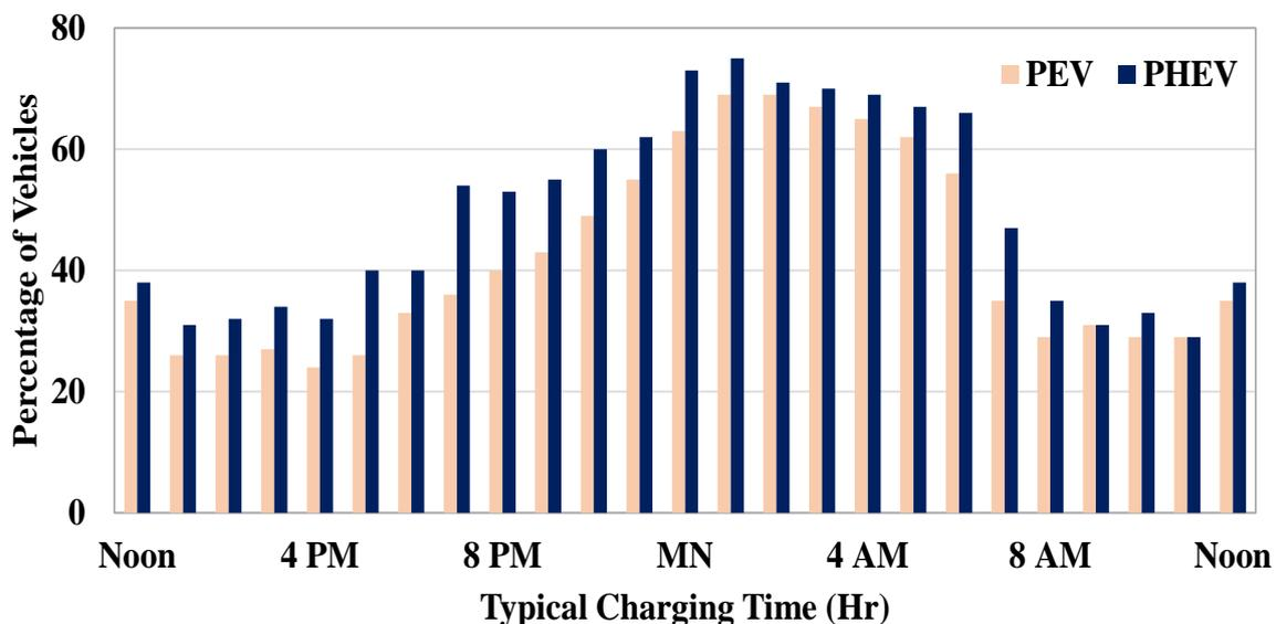
**Figure 8.** Residential Electric Vehicles charging times, California Vehicle Survey, May 2018.
