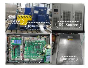
Figure 12. Photo of the experiment system.
