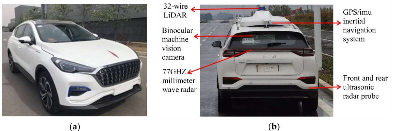
Figure 10. Experimental vehicle configuration: (a) experimental vehicle; (b) sensor locations.
