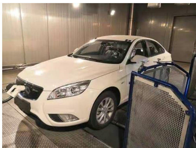
Figure 5. Drum test of a test car in the laboratory.
