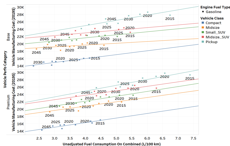
Figure 15. Manufacturing cost versus fuel consumption of split HEVs.
