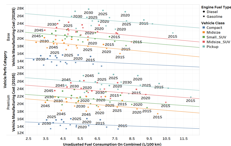
Figure 14. Manufacturing cost versus fuel consumption of conventional vehicles.
