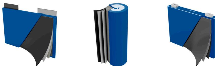
**Figure 1.** Typical Cell Types for Lithium Ion Batteries. From left to right: Pouch Cell, Cylindrical Cell and Prismatic Cell.
