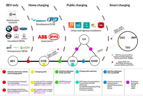
BEV: Battery electric vehicle EVSE: Electric vehicle supply equipment CPO: Charge Point Operator EMSP: Electric mobility service provider CH: Clearing House DSO: Distribution service operator TSO: Transmission service operator BRP: Balance Responsible Partv
