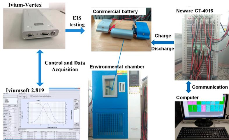
Figure 1. Battery test platform.
