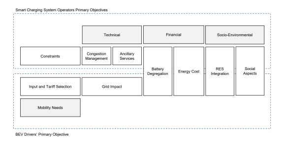
Figure 2. Objectives of Smart Charging System Operators and BEV Drivers.
