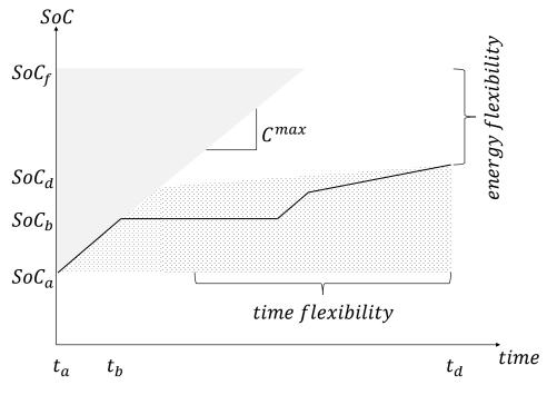
Figure 1. Schema for charging flexibility.
