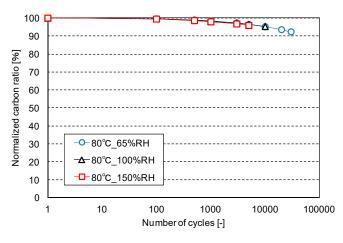
**Figure 7.** Effect of humidity on the relationship between the normalized carbon support corrosion ratio and the number of potential cycles.
