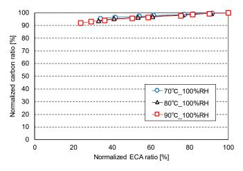
**Figure 4.** Effect of cell temperature on the relationship between the normalized ECA ratio and the normalized carbon support corrosion ratio.
