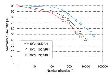
**Figure 6.** Effect of humidity on the relationship between the normalized ECA ratio and the number of potential cycles.
