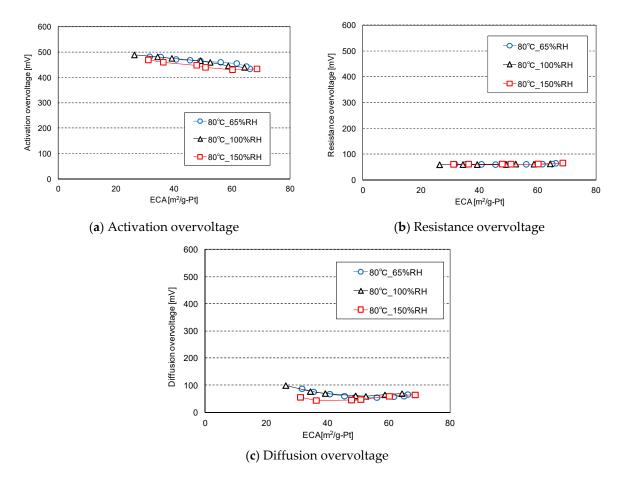
**Figure 11.** Effect of humidity on the relationship between overvoltage and ECA at a current density of 1 A cm<sup>-2</sup> during the load cycle test.
