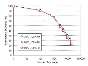
**Figure 2.** Effect of cell temperature on the relationship between the normalized ECA ratio and the number of potential cycles.
