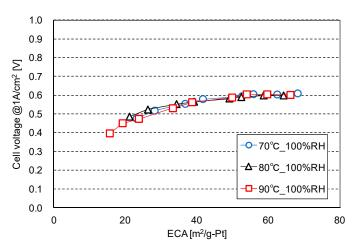
**Figure 5.** Effect of cell temperature on the relationship between the cell voltage at  $1 \text{ A cm}^{-2}$  and the ECA in the load cycle durability test.
