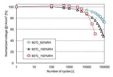
**Figure 10.** Effect of humidity on the relationship between the cell voltage at  $1 \text{ A cm}^{-2}$  and the number of potential cycles.
