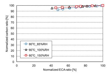
**Figure 8.** Effect of humidity on the relationship between the normalized ECA ratio and the normalized carbon support corrosion ratio.
