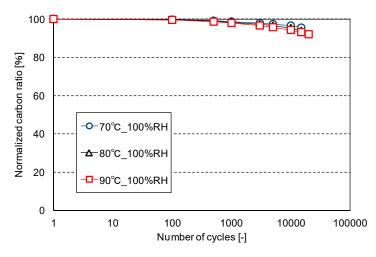
**Figure 3.** Effect of cell temperature on the relationship between the normalized carbon support corrosion ratio and the number of potential cycles.
