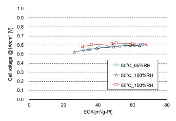
**Figure 9.** Effect of humidity on the relationship between the cell voltage at  $1 \text{ A cm}^{-2}$  and the ECA in the load cycle durability test.
