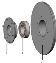
**Figure 10.** Assembly drawing of wheel hub. 1—bearing cap, 2—bearing, 3—end cap.
