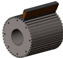
**Figure 7.** Connection diagram of single-tooth and core skeleton.
