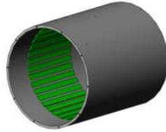
**Figure 9.** Assembly drawing of magnetic poles and rotor core.
