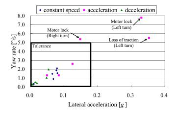
Fig. 7(b) Motor malfunction of the fourth axle on the right without redundancy control
