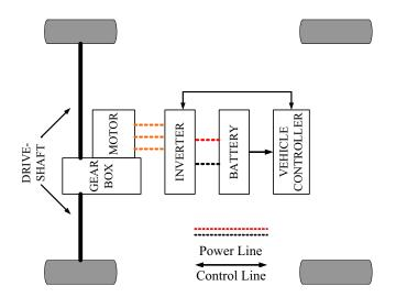
Fig. 3 Block diagram of drive system of conventional EVs (Front-wheel drive)
