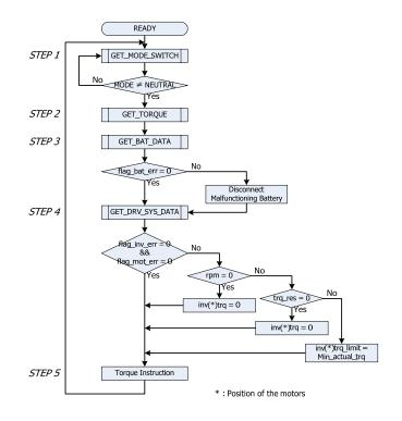
Fig. 5 Flow chart of redundancy control
