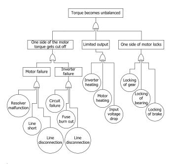
Fig. 2 Fault tree analysis of the phenomena that lead to unbalanced traction forces
