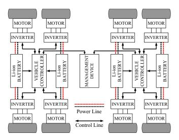
Fig. 4 Block diagram of Eliica's drive system with redundancy (All-wheel drive)
