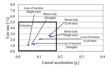
Fig. 8(b) Motor malfunction of the fourth axle on the right with redundancy control
