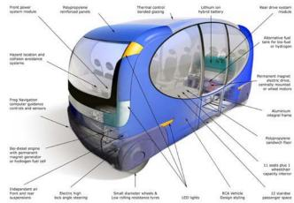
Fig. 15 Cutaway view of latest vehicle design
