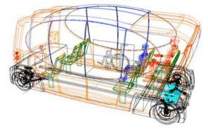
Fig. 6 3D packaging design of virtual prototype
