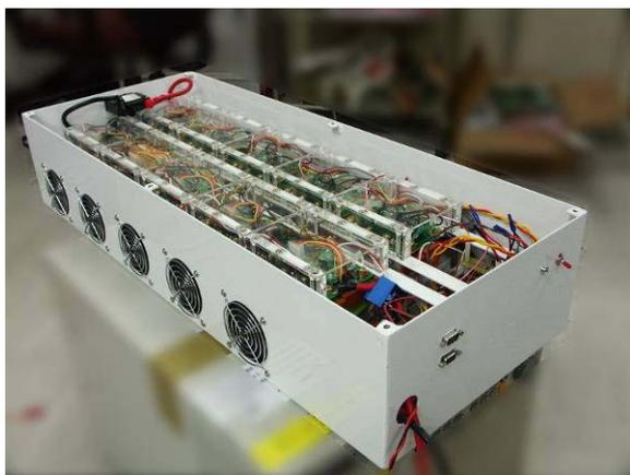
Fig. 6 Appearance of 144V Lithium-ion battery energy system
