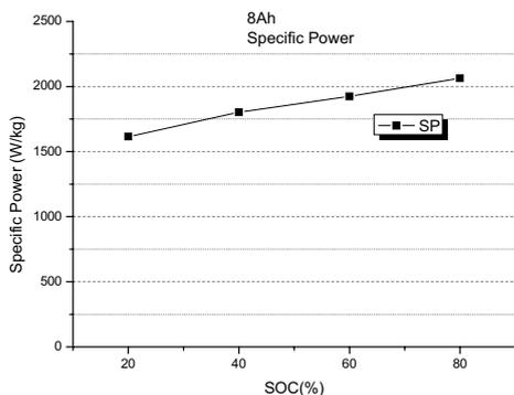
Fig. 3 Specific power characteristic of 8Ah Lithium-ion cell
