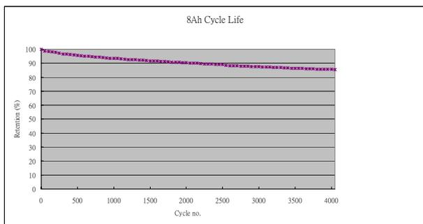
Fig. 4 Cycle life characteristic of 8Ah Lithium-ion cell (charge and discharge at 60%-80% SOC)
