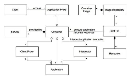
Figure 6. Class diagram of the container pattern.
