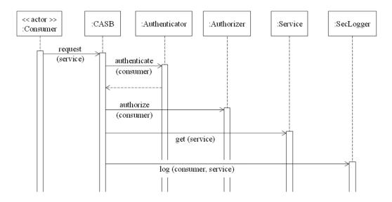
Figure 4. Sequence diagram for the use case "Access an application service".
