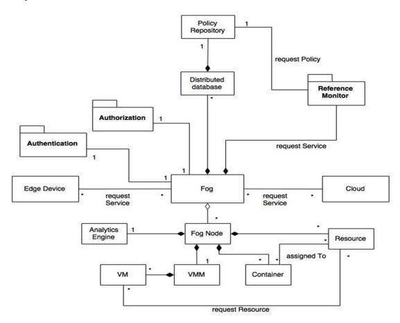
Figure 7. Class diagram of the Fog Computing pattern.
