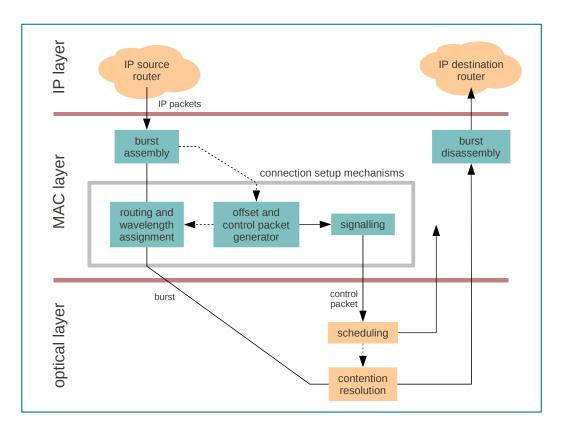
Figure 2. Functional block diagram of IP over OBS (adapted from [20]).
