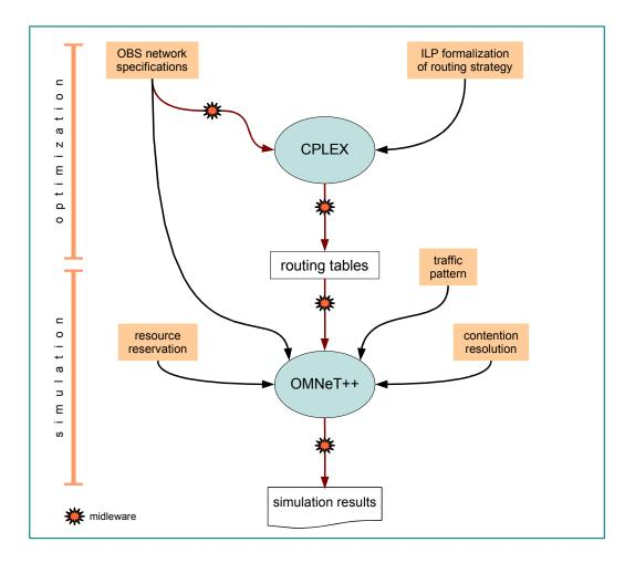
Figure 6. Conceptual view of the simulation methodology.
