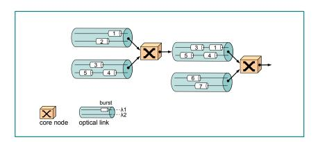
Figure 10. An illustrative example of the streamline effect.
