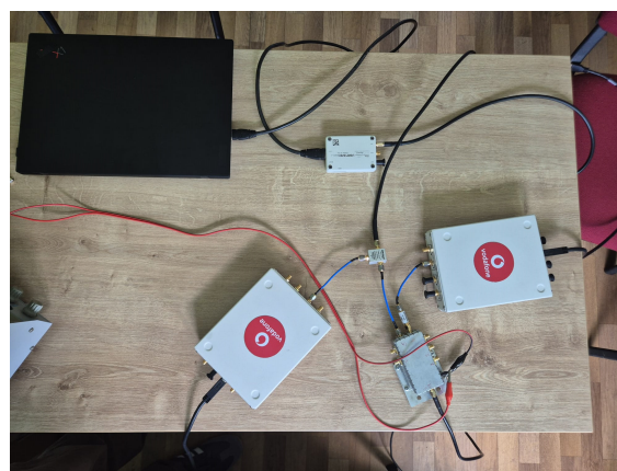
Figure 6. Cable-coupled jamming setup for USRP B210 receiver: two USRP B210 units (left), one connected directly to the main splitter (bottom) and one connected through a secondary splitter combining the antenna feed with the jammer noise injected over a cable path (top); the jammer's own USRP B200mini and dedicated laptop are visible on the right.
