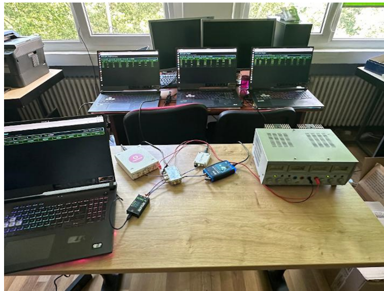
Figure 4. Picture of the measurement setup including four different SDR platforms.
